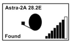
Here we have found the satellite, make small adjustments to the dish and LNB to maximize your signal.
